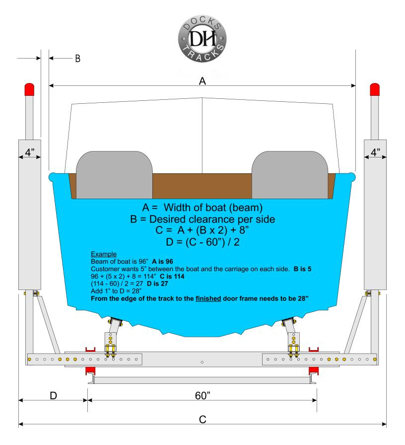
If the track is not going to be centered in the doorway, use this formula to determine the distance from the edge of the door to the edge of the track . You should add one inch to the 'D' dimension for clearance between the door opening and the carriage.
