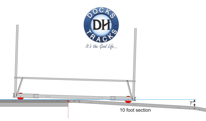
The first section out the cement slab can only drop 7 inches in 10 feet or 3-1/2 inches in 5 feet. This is to prevent the carriage from dragging on the edge of the slab as it makes it's descent. If 10 feet out is too far to begin descending into the lake, a 5 foot section can be used. This will allow a more rapid descent closer to the doorway. Keep in mind; the maximum descent is 2 feet for every 10 feet of track.
